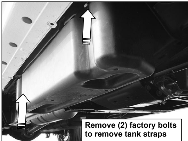
(Fig 9) Passenger side DEF tank and cover
