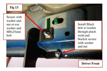
**Step 7:** Middle Driver will install the same as the front it will use (2) bolts in the pinch weld. Snug all fasteners to hold bracket but do not tighten.
