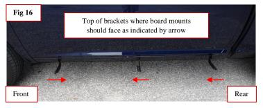
**Step 9:** Now install running boards on the brackets. Obtain the bracket to board bolt pack. Take out the provided 5/16<sup>\*\*</sup>3/4<sup>\*</sup> bolts. Slide the head of the bolts down the channels on the underside of the board.
