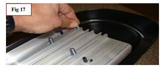
**Step 14:** Place the board on the installed mounting brackets. Align the bolts with the slots on the brackets and drop them into place. Next thread the provided 5/16" flange nuts onto the bolts to hold the board and leave loose. Adjust the board in or out, right or left to meet your needs. Once the boards are in place to your liking, tighten all fasteners on the brackets. Front and rear first and then the center brackets finally the boards. This will complete your installation. Enjoy!
