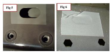
**Step 3:** We need to remove the factory tape at each location. Peal it off and keep it clean. It can be put back to its original place after the bolt plate is installed.
