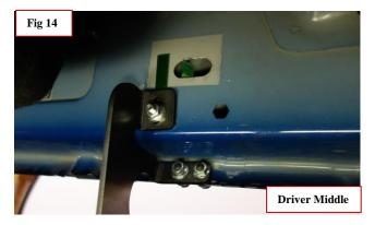
**Step 8:** Rear Driver will install the same as the front and middle brackets. It will use (1) bolts in the pinch weld. Snug all fasteners to hold bracket but do not tighten.
