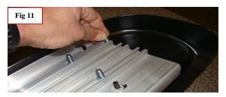
**Step 9:** Place the board on the installed mounting brackets. Align the bolts with the holes on the brackets and drop them into place. Next thread the provided 5/16" flange nuts onto the bolts. Do not tighten. Adjust the board in or out, right or left to meet your needs. Once the boards are in place to your liking, tighten all fasteners on the boards and brackets. This will complete your installation. Enjoy!
