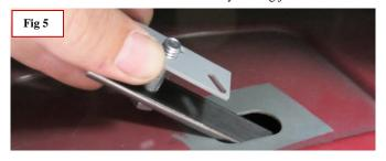
**Step 6:** Make sure when bolt plate is installed that it is not standing up on bottom ledge inside cavity. This will allow the bolt not to rest on the lower edge of the slot and cause the bracket to be mounted to high. Installed properly the stud should be resting on lower edge of oval hole as shown (Fig 6). Now install (2) 3/8" washers over stud to compensate for recess in body panel.
