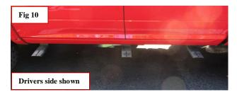
**Step 8:** Now install running boards on brackets. You may have different boards than shown. However, they will have the same type of mounting unless additional installation instructions are provided. Obtain the bracket to board bolt pack. Take out the provided 5/16"\*3/4" bolts. Slide the head of the bolts down the channels on the underside of the board.
