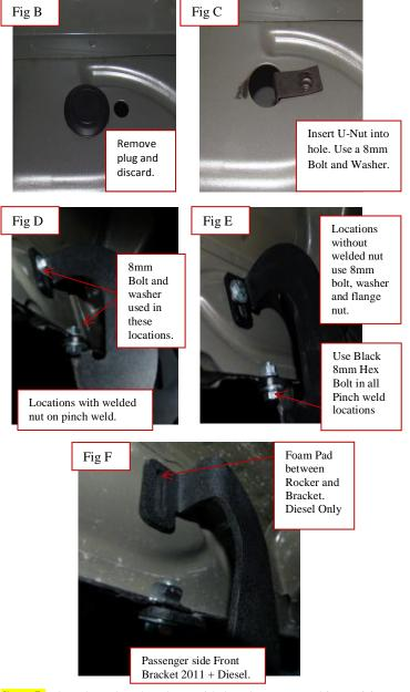
**Step 5:** Place board on brackets with bracket mounted in position. Look on underside of board to which channel will match up with bracket slots to slide the 5/16" bolts down on the underside of board so bolt stud will be lined up with bracket slot. You will only need one bolt to secure board to each bracket. Two bolts per bracket are supplied if applicable. Loosely hand-tighten 5/16" nuts to hold board to brackets.
