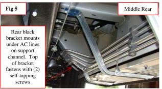
Step 4: When brackets are mounted in position and board is supported in installed location, snug board bolt making sure brackets are vertically lined up with support rails. Screw (2) self-tapping screws into holes in top of bracket into support rails at each bracket location.
