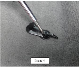
2) WITH THE FACTORY CLIPS REMOVED, UNSCREW THE TWO HALVES OF THE HUSKY® RETAINING CLIP AND INSERT THE BOTTOM HALF INTO THE EXISTING FACTORY GROMMETS LOCATION AS SHOWN BELOW IN IMAGE 5 AND IMAGE 6. THE BOTTOM PORTION WILL "SNAP" SECURELY INTO THE FACTORY GROMMET LOCATION. RETAIN THE TOP HALF OF THE CLIP FOR LATER INSTALLATION.
