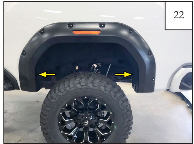
Install (2) panel retainers (RV1-P008).
