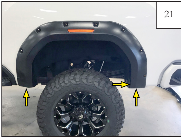
Reinstall (3) T-15 torx screws.
