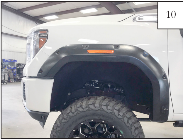
Completed front flare installation.
