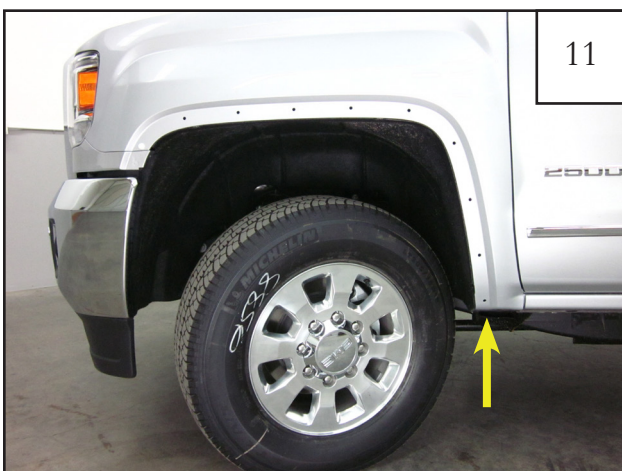
Reinstall factory fastener removed in step 6 using a 1/2" socket and wrench.
