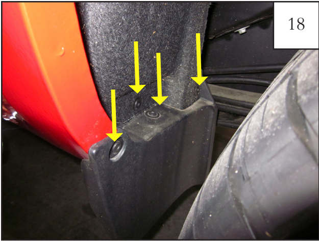
Using a T-15 Torx bit socket wrench, remove the four factory screws from the factory forward splash guard. Remove splash guard and discard.
