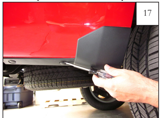
Using a pry tool, remove factory retainers in bottom of factory rear mudguard. Remove mudguard and discard.
