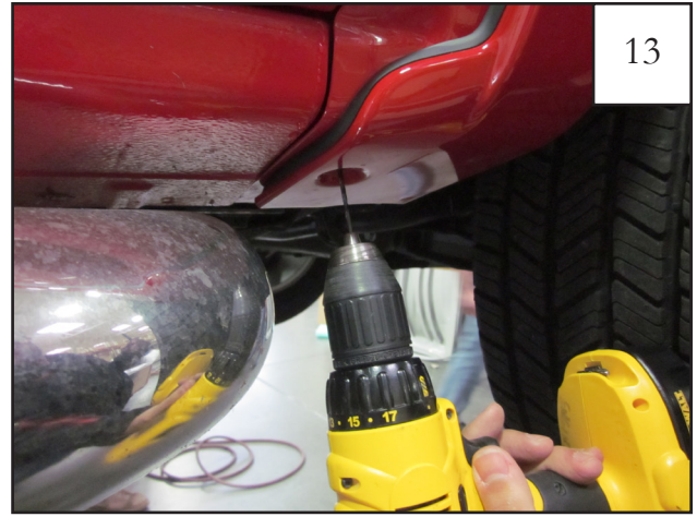
Using a 3/32" drill bit, drill bottom fastener location marked in step 9.
