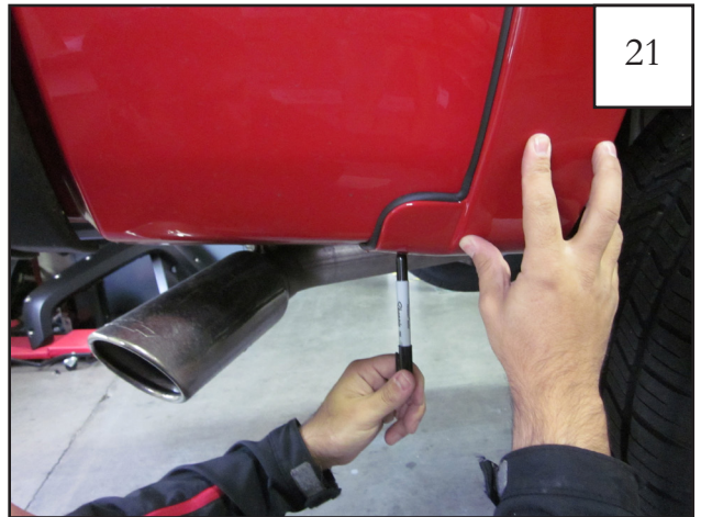
Using a grease pencil, mark the rear bottom fastener using the flare as a guide.
