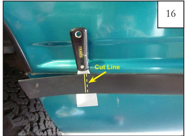
Slide putty knife between the molding and the body of the vehicle.
