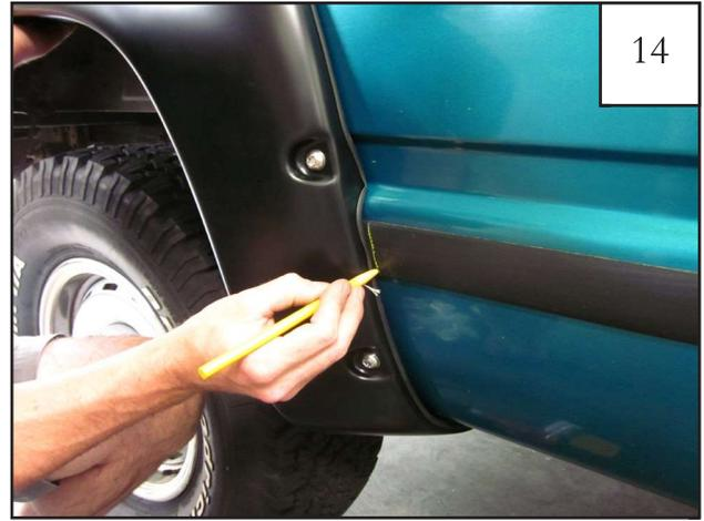
The factory installed body side molding (when present) will need to be trimmed to allow the flare to lay flush against the sheet metal. Hold the flare up to the wheel well opening and mark a line on the body side molding where the flare overlaps it.
