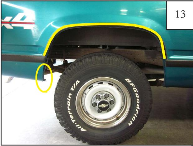
Remove factory fender trim and mud flaps (when installed).
