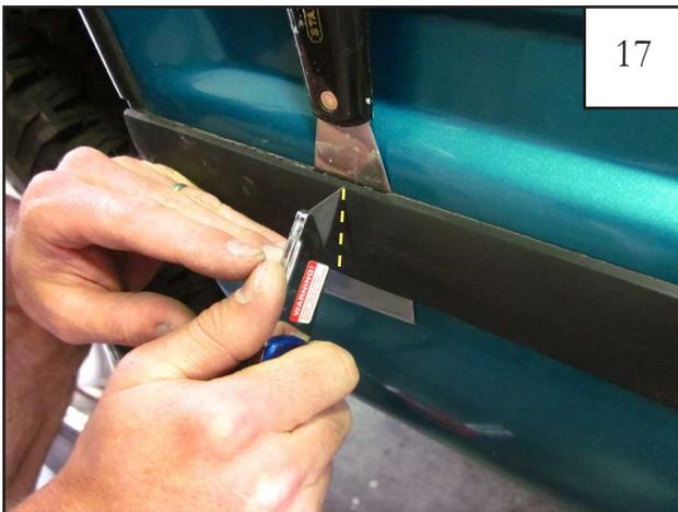
Carefully cut on marked line with a utility knife, using the putty knife as a guard against the vehicle. Sand molding to desired finished edge.
