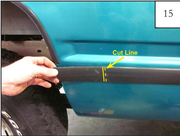
Remove the flare and mark a cut line 1/4" beyond overlap line. Use blow dryer or heat gun to heat molding.
