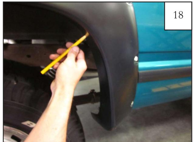
Hold flare in position on fender using moderate pressure. Using a grease pencil, mark five hole locations using the holes in the flare as a guide. (See Step 19)
