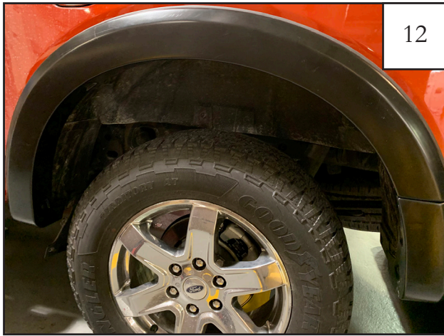
Align fender flare with holes and position on fender.
