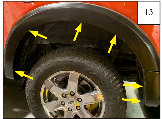
Install (6) RV1-P018 fasteners.
