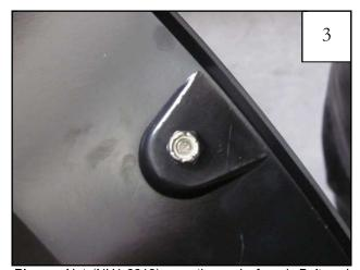
Place a Nut (NU1-0019) over the end of each Bolt and tighten, using a 1/2" wrench for the Nut and the supplied Torx Bit (SW1-0052) for the Bolt.
