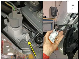
Squeeze the lower tab on the back of the turn signal assembly and remove from the truck. Carefully turn the wiring harness counter-clockwise and separate the bulb/wiring harness from the turn signal assembly.
