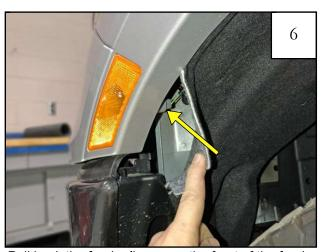
Pull back the fender liner near the front of the fender and locate the turn signal assembly and wiring.
