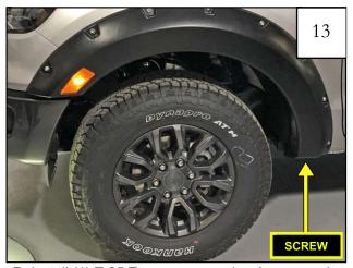
Reinstall (1) T-25 Torx screw previously removed from rear of the flare in Step 5.
