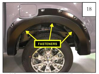
Hold flare to vehicle and install (3) 1/4" panel retainers (RV1-P008) into the wheel well holes indicated. Press firmly on the flare while installing fasteners.
