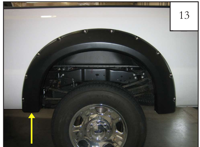
13 Place flare on fender and reinstall bolt removed in Step 8.
