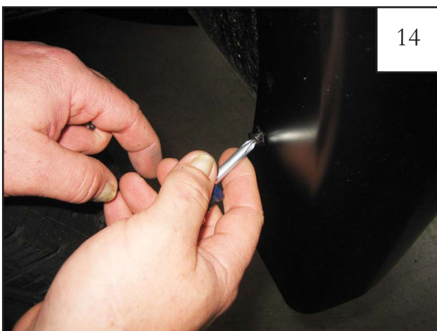
14 Install four supplied Screws (SW1-0050) through remaining holes and into clips installed in Step 12, working from front to back of wheel well.
