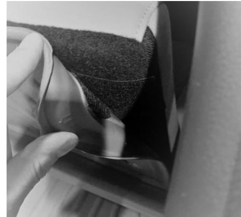
4. Install the liner as shown. Before installing, fold the 3<sup>rd</sup> row seat flat. Next, position the liner in the portion of the cargo area behind the wheel wells, then extend the liner over the backs of the stowed 3<sup>rd</sup> row seat. You may need to press the liner down to fully seat the Velcro pads in place.
