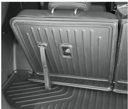
6. The liner at this point is fully installed and is ready to use. If the liner needs to be removed, grab the rectangular Velcro patches and hold them firmly in place as you pull the liner from the seat. This Velcro piece is intended to stay attached to the seat back and cargo floor to reduce ware from the liner being installed and reinstalled for cleaning.
