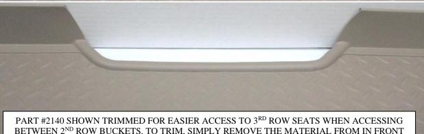
PART #2140 SHOWN TRIMMED FOR EASIER ACCESS TO 3<sup>RD</sup> ROW SEATS WHEN ACCESSING BETWEEN 2<sup>ND</sup> ROW BUCKETS. TO TRIM, SIMPLY REMOVE THE MATERIAL FROM IN FRONT OF THE RAISED MOAT USING THE FRONT EDGE OF THE MOAT AS A TRIMMING GUIDE. CONTINUE TRIM UP AND THROUGH THE FRONT WALL OF LINER.
