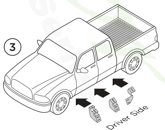
**4.** Align the Front, Center and Rear Driver's Side Brackets with the indicated holes located on the Rocker Panel of the vehicle.
