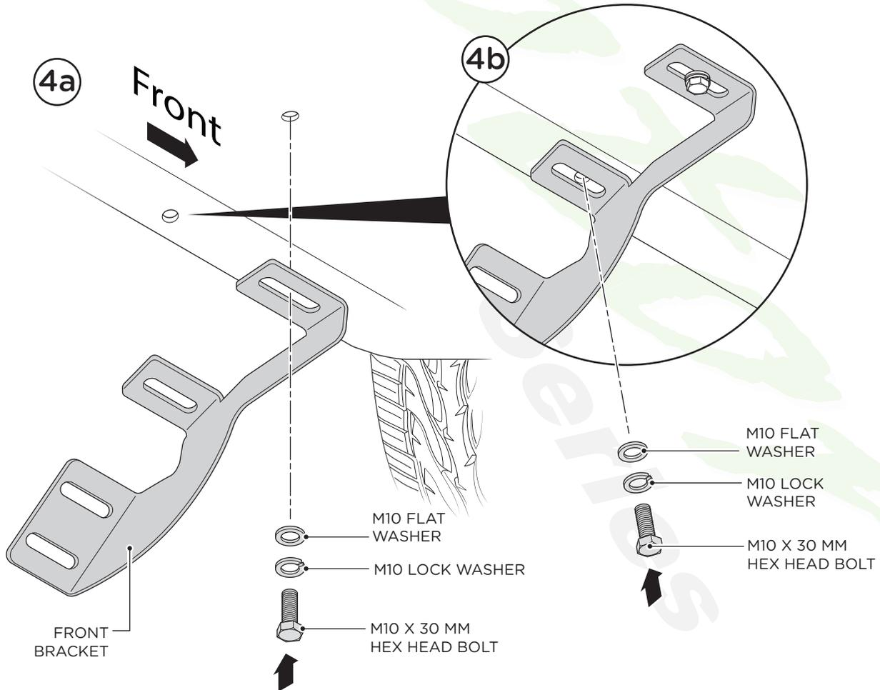
5. Fasten each bracket using two (2) M10 x 30MM Hex Head Bolts, two (2) M10 Flat Washers, two (2) M10 Lock Washers.
