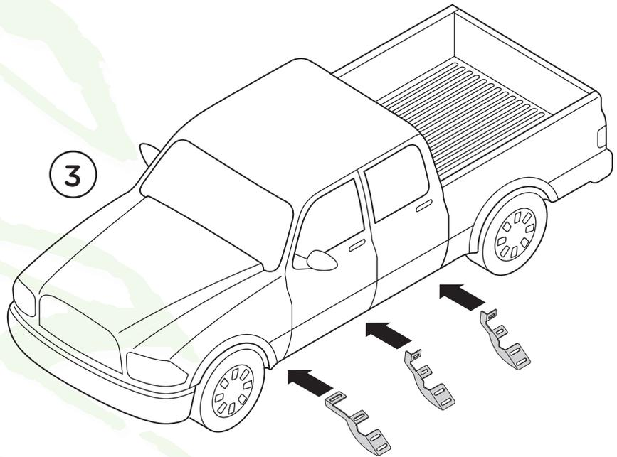
**4.** Fasten each bracket using two (2) M10 x 30MM Hex Head Bolts, two (2) M10 Flat Washers, two (2) M10 Lock Washers.
