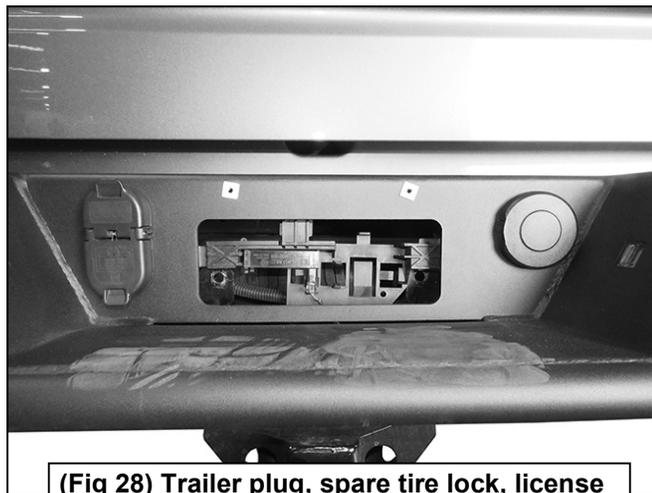
(Fig 28) Trailer plug, spare tire lock, license plate plugs and TPMS antenna installed
