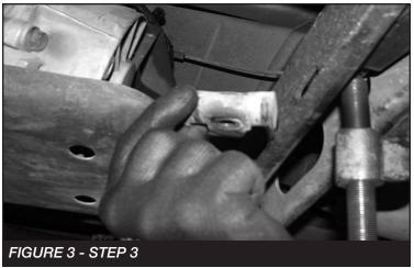
Carefully unload the torsion key and tool. Next, slide the torsion bar forward (note the key clocking position) then remove the factory torsion key. SEE FIGURE 4
