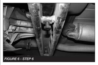
Remove the lower shock bolt. Save for reinstallation. SEE FIGURE 7
