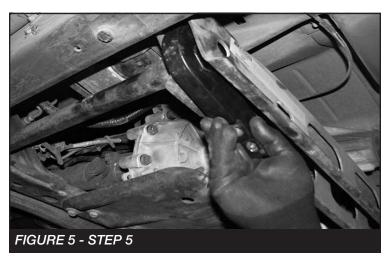
Reinstall the torsion key tool and adjust upward enough to reinsert the adjustment block. Remove the tool and install the factory bolt so that it is flush with the bottom of the crossmember. SEE FIGURE 6
