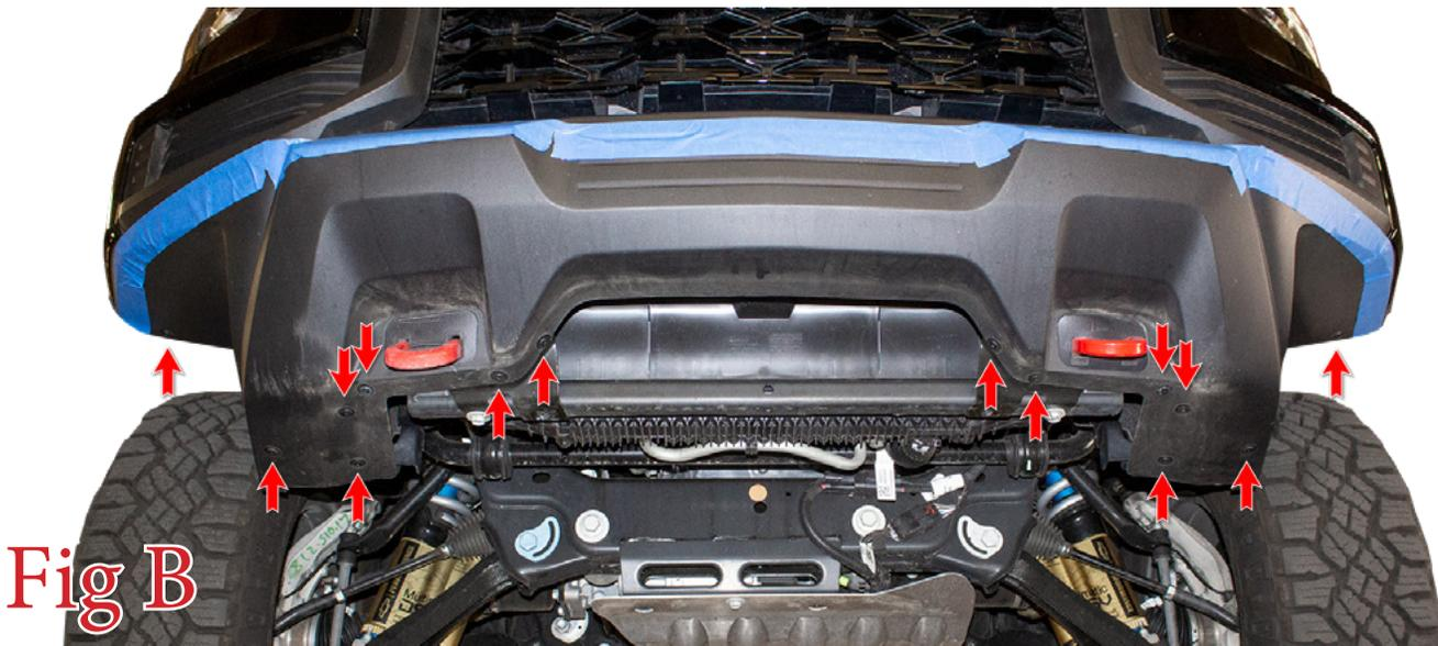
3. Inside each wheel well, use a T-15 Torx Socket to remove the 3 lower inner fender liner bolts. Then remove the 7mm bolt referenced in (Fig C).
