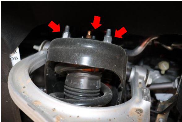
9. Remove three 18mm top hat nuts.
