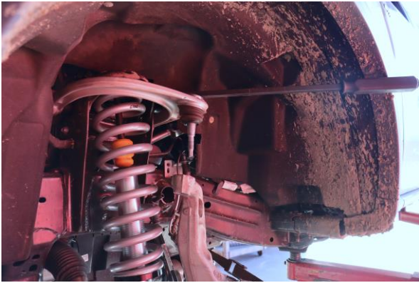
15. Use a pry bar to pull down on the upper control arm. Lower the upper ball joint into the top of the steering knuckle and install the upper ball joint nut hand tight.
