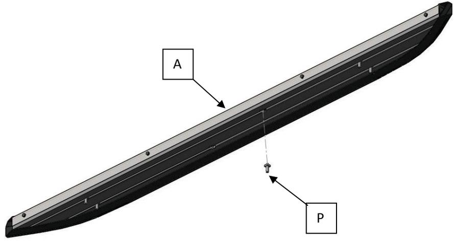
**2** Locate the existing hole locations shown below. There will be two sets of hole locations (Front, Rear). Remove any plastic plugs in the locations
