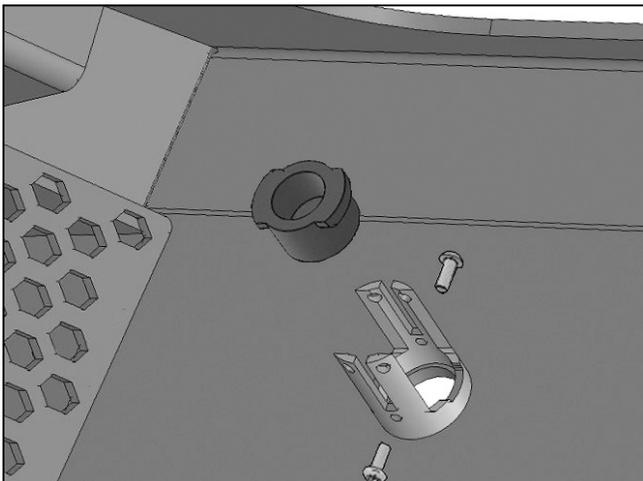
(Fig 5) Push Rubber Plug into sensor mounting sleeve. Use 4mm Screws to lock plugs in place.
