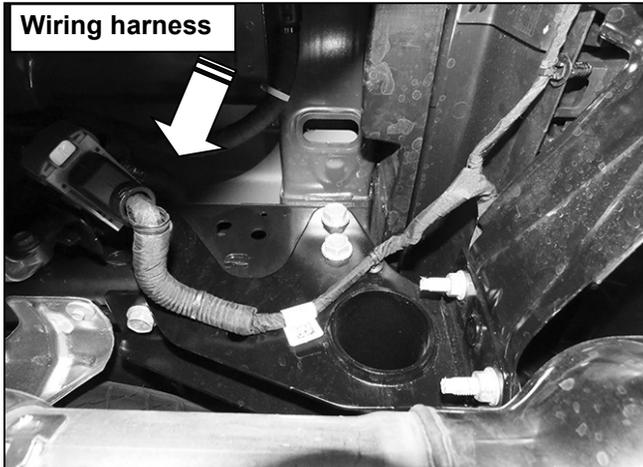
(Fig 1) Unplug wiring harness leading to bumper
