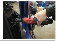
Gently unclip one reflector on each side of the rear fascia to access and remove one fastener on each side using an 8mm socket.
