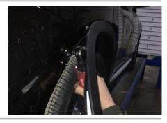
Remove one plastic clip on each side using a pry tool. Gently unclip the plastic covers located on the inside of each taillight.
