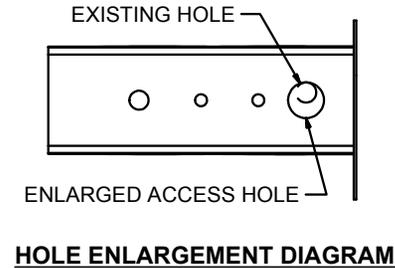
2. On the driver side, fishwire a 7/16" carriage bolt and SP2 spacer through the enlarged access hole and out the forward most mounting hole. Reverse fishwire a 7/16" carriage bolt and SP2 spacer in the enlarged access hole. On the passenger side, fishwire 7/16" carriage bolts and SP2 spacers through the existing access hole and out the mounting holes. See Fishwire Technique Diagrams.
