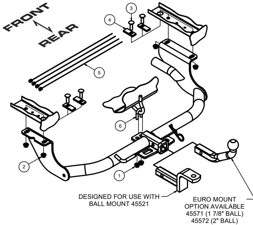
1. Enlarge the existing hole on the driver side to allow 7/16" carriage bolts and SP2 spacers to pass through. See Hole Enlargement Diagram.
