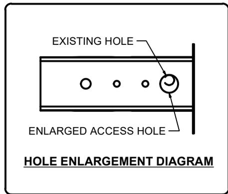
2. On the driver side, fishwire a 7/16" carriage bolt and SP2 spacer through the enlarged access hole and out the forward most mounting hole. Reverse fishwire a 7/16" carriage bolt and SP2 spacer in the enlarged access hole. On the passenger side, fishwire 7/16" carriage bolts and SP2 spacers through the existing access hole and out the mounting holes. See Fishwire Technique Diagrams.
