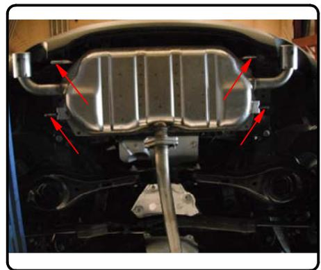
2) Remove the tape if present from the forward most attachment point and fishwire the (2) supplied carriage bolts and (2) sp-6 spacers on both sides. Reverse pull the remaining (2) bolts and (2) spacers on both sides into the rearward attachment holes. Leave the wires on temporarily while raising hitch (refer to diagrams to the left for fishwiring techniques).
