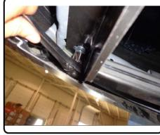
5. Torque all 7/16" hardware to 59 ft-lbs. Torque all 8mm hardware to 23 ft-lbs.
