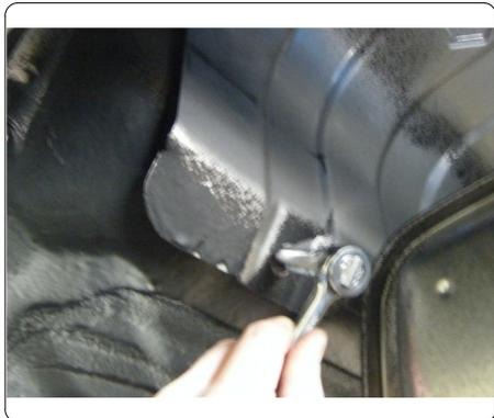
8. Install 1/2-13 carriage bolt and CM-SP4 spacer through top of existing vehicle tow loop, as shown.
