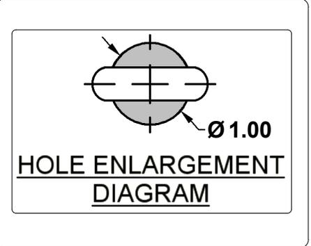
6. Reverse fishwire 1/2-13 carriage bolts and CM-SP6 spacers through the enlarged access hole, both sides.
