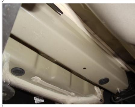
4. Locate and remove rear rubber cap from driver and passenger side frame rail.
