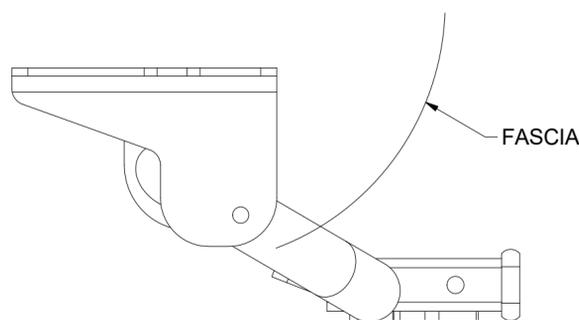
INSTALLED HITCH POSITION
