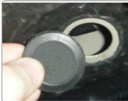
5. Enlarge driver and passenger side mounting holes enough to allow 1/2-13 carriage bolts and CM-SP6 spacers to pass through. (SEE HOLE ENLARGEMENT DIAGRAM.) **NOTE:** Korean built models only. Raise hitch into position using hitch as a template, mark and drill holes large enough to allow 1/2-13 carriage bolts and CM-SP6 spacers to pass through. Coupe models: Also enlarge 1/4" hole to allow for 1/2" carriage bolt.
