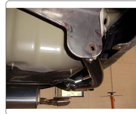
10. Loosely install 1/2-13 flanged nut onto carriage bolt from both frame rails.
