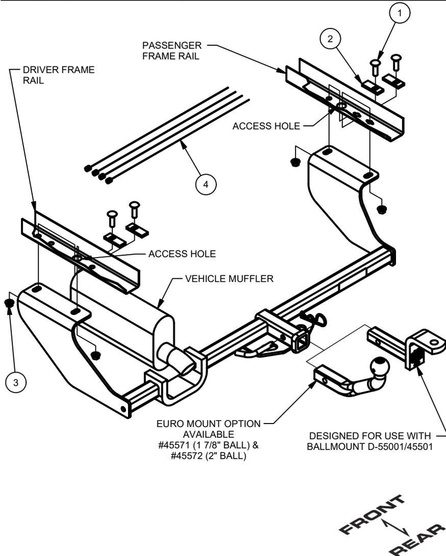
1. Fishwire CM-SP2 spacers and 7/16-14 carriage bolts through access holes and into attaching holes. Leave fishwires attached.
