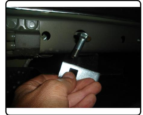
2. Raise hitch into position, being careful not to push bolts back into frame.
