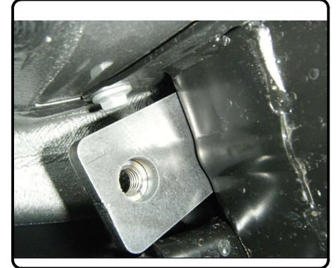
6. Seal around the back two holes on hitch with silicone caulk. Raise hitch into position, aligning the slots in the hitch with the holes in the nut plates.
