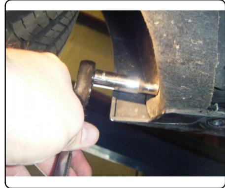
2. Remove (2) 12mm nuts from each bumper attachment. These will be re-used in STEP 4.
