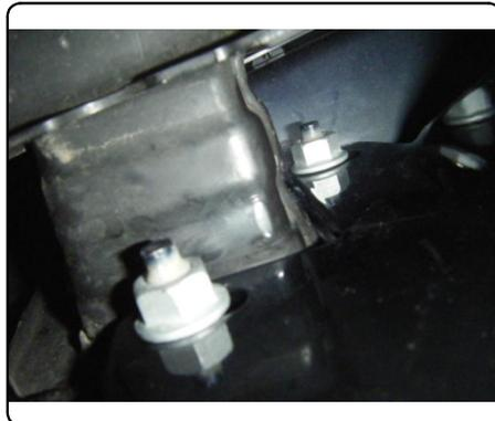
5. Fishwire 1/2" carriage bolts and SP-6 spacers into vehicle crossmember. (See FISHWIRE TECHNIQUE below) Note: If holes are not present, use mounting strap as a template to mark & drill 17/32" holes.
