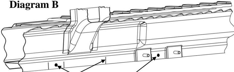
Marked vertical line that was transferred from Diagram A to the inside of the rocker panel.
