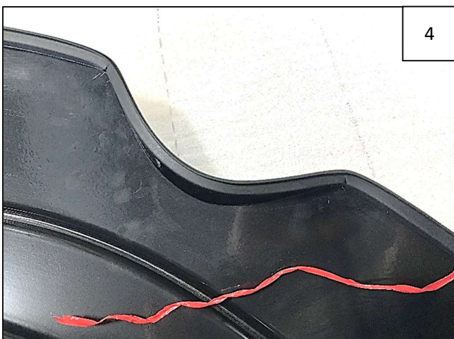
Correctly-installed edge trim around gas door.
