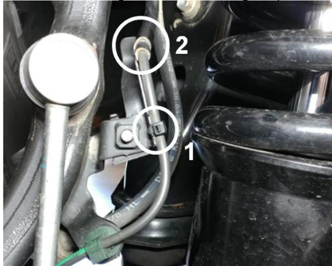
II. Remove OE ABS line bracket by removing the hex head cap screw with a 10mm socket. Note: picture is of non-KDSS 4Runner model, disregard sway bar end link.
