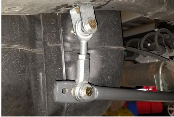
21. Adjust the length of the end links to set the sway bar as parallel with the ground as possible, while still having at least 7-8 turns of thread on the Heim joint remaining.
