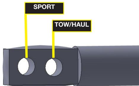
16. Attach the end links onto the Belltech bar using the original 18mm nuts. Torque to 16 ft lbs. once the vehicle is back on the ground.
