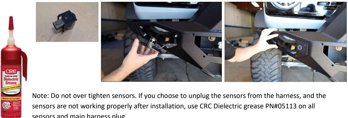
Note: Do not over tighten sensors. If you choose to unplug the sensors from the harness, and the sensors are not working properly after installation, use CRC Dielectric grease PN#05113 on all sensors and main harness plug.
