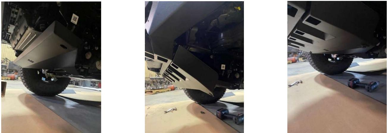
3. Plug the sensors into the harness on the front winch cover plate and install to the bumper. Then install 1/4"-20 cage nuts onto the mesh bolt in plates and install the plates on each side of the bumper.
