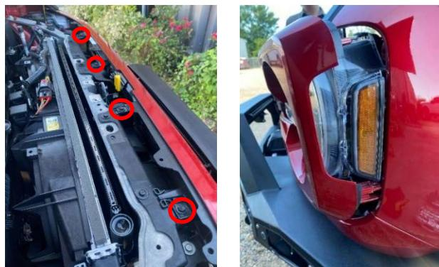
3. Now that the grill is free, disconnect your camera and camera washer spray line, above your passenger headlight. Once those items are disconnected, remove grill and set aside. Uninstall your camera from the grill and remove the factory camera harness and the sprayer tube. **(Washer spray tubing will need to be capped or plugged: plug with a 1/4" bolt and zip tie)**
