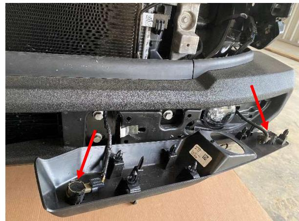
2. Once the plastic covers are removed, (a) locate the front sensor harness plug behind the driver side headlight and fender liner, (b) and unplug the harness. Now remove the 6 frame bolts using an 15mm socket, and the front bumper will come off.
