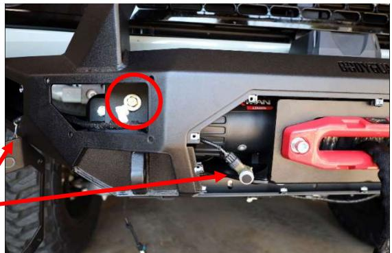
4. Adjust fitment vertically and horizontally using a tape measure, then tighten hardware.
