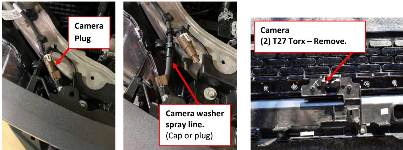
1. Reconnect the camera harness that you removed from the grill to the connector above your headlight. Run the harness down between the core support and your headlight. Attach the provided **89758 camera harness** to the factory harness. Once the Bodyguard bumper is installed the excess camera harness will run through the cutout in the baja bar up to the camera.
