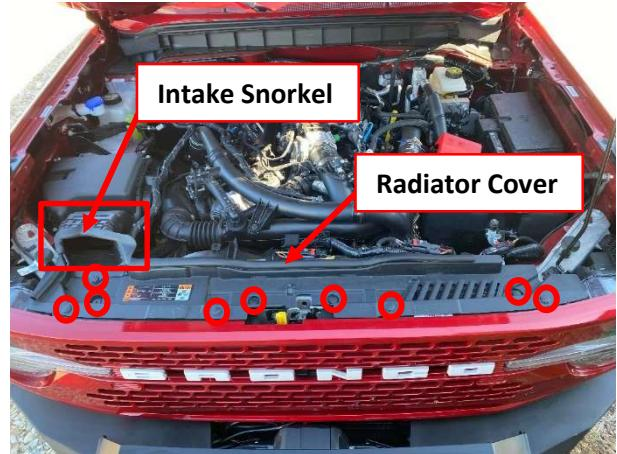
2. Once the radiator cover has been removed, remove the (4) bolts using a 10mm socket holding the top of the grill. Pry gently at the top corners of the grill and work your way around the bottom and pull outwards. Until the grill is free to be removed.
