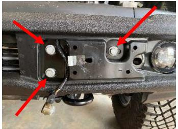
3. Once the bumper is off, detach the parking sensor wiring harness from the bumper, and locate the (6) bolts holding the skid plate, then remove the skid plate using the 15mm socket. With the skid plates off, remove both tow hook shrouds by sliding forward.
