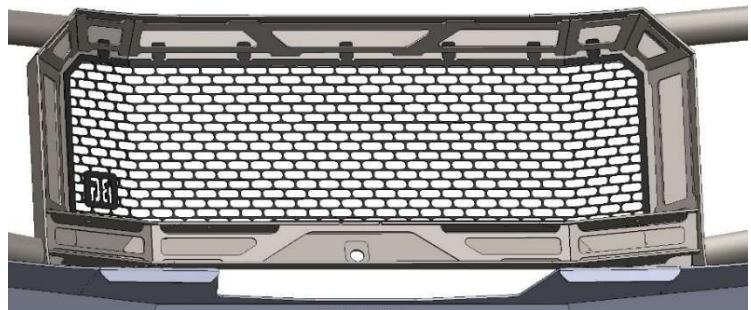
3. Install the mesh by sliding the top tabs under the webbing on the Extreme Guard. Once the tabs have are slid into place, bolt the mesh in place using the provided 1/4"-20 hardware. (If you have Adaptive Cruise Control, you will want to leave the two driver side bolt locations open.)
