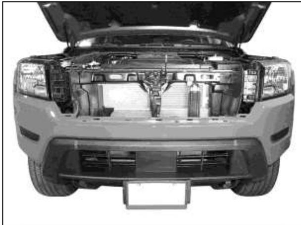
(Fig 8) Remove factory grille assembly
