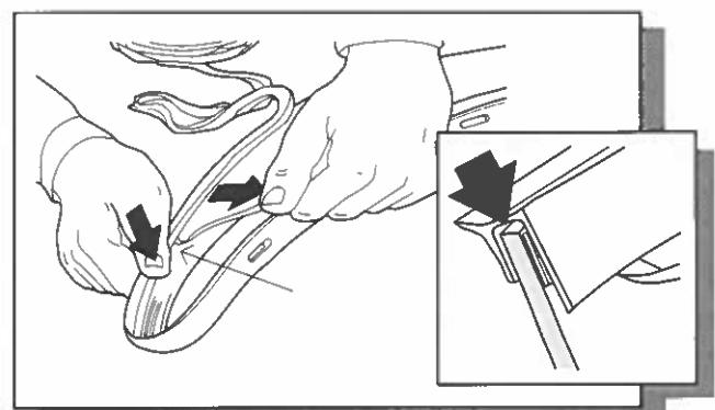
4. Remove approximately 2" (50mm) of the protective liner from the extrusion. Fit the extrusion to the Fender Flare along the edge that comes in contact with the vehicle's body panel.
