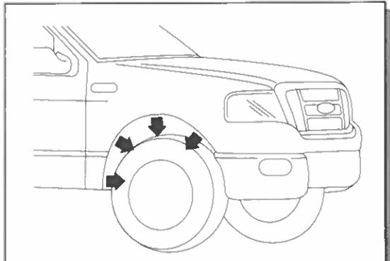
10. Remove the previously noted existing screws and retain for re-installation.
