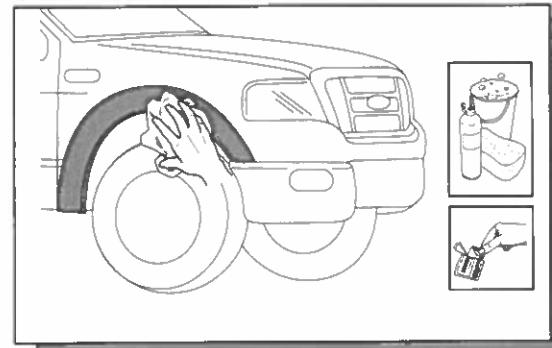
3. Wash the areas of contact on the vehicle and wipe dry both the vehicle and the Fender Flares with a clean cloth. Ensure inside of Fender Flares where extrusion is attached is clean, use alcohol wipe supplied to clean surface.
