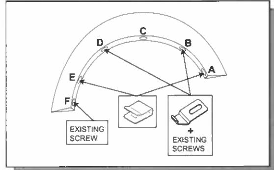
7. Note the correct hardware for positions **A**, **B**, **D**, **E** & **F** (Right Fender Flare shown).
