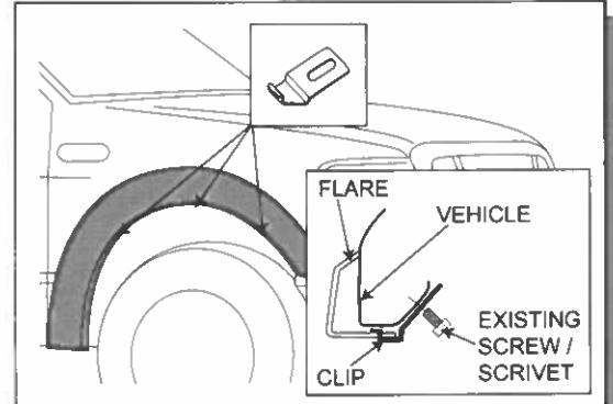
11. Place Fender Flare on the vehicle. Using the lever clips provided, install them into positions **B**, **C** and **D**, by locating the leg of clip into slot in Fender Flare and then secure clips to vehicle using the previously removed screws or scrivet for 2007-on models as shown.
