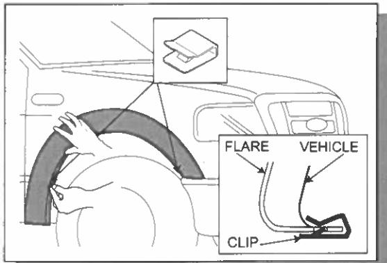
**12.** Take the supplied snap clips and fix them into positions **A** and **E**, as shown, ensuring the notch in clip locates securely into the slot in the Fender Flare.
