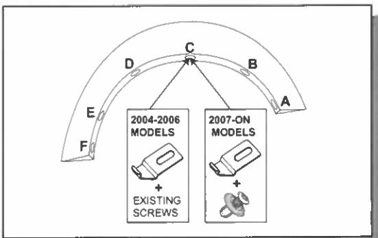
8. Note the correct hardware for position **C** (Right Fender Flare shown).
