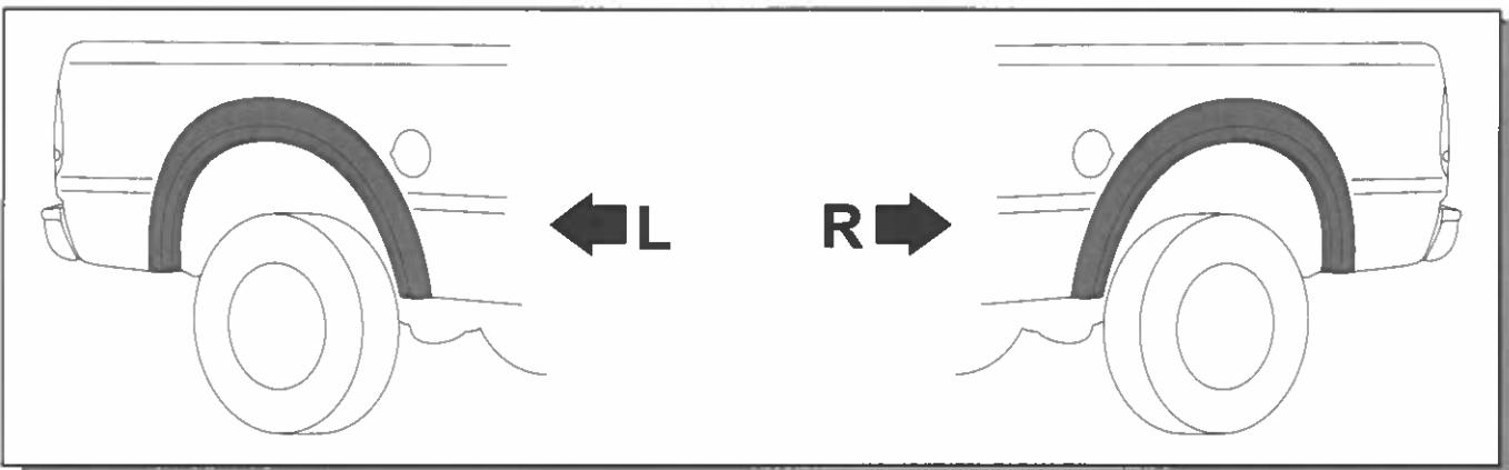
1. Ensure that both left and right hand Fender Flares suit the profile of the vehicle. Note the areas where the Fender Flares come in contact with the vehicle. **NOTE:** Before fitting Fender Flares remove any mouldings, strips or existing flares from the wheel arch. If there is a body side moulding, mark where the moulding is to be cut, alternatively the Fender Flares can be cut to go around the moulding. Be sure to allow enough room for the extrusion.
