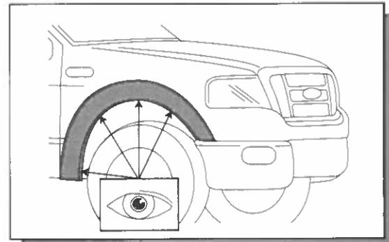
9. Place the Fender Flare on the vehicle into the position of best fit. Note where the slots in Fender Flare at positions **B**, **C**, **D** and **F** align with the existing screws in the vehicle. Remove Fender Flare.
