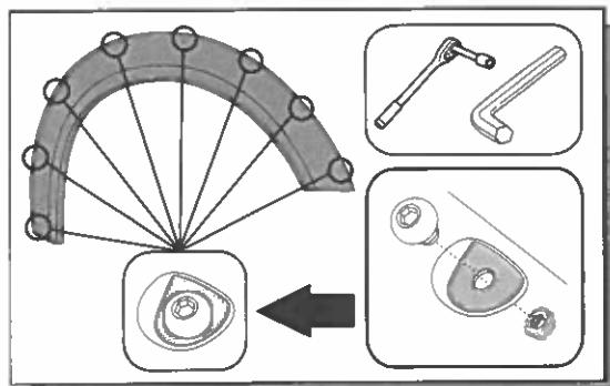
2. Attach 9 bolts to each Fender Flare using a 3/16" Allen key and a 1/2" wrench/socket. (socket wrench and Allen key not supplied)
