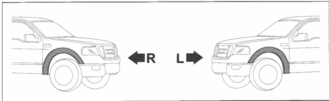
1. Ensure that both left and right hand Fender Flares suit the profile of the vehicle. Note the areas where the Fender Flares come in contact with the vehicle. **NOTE:** Before fitting Fender Flares remove any mouldings, strips or existing flares from the wheel arch. If there is a body side moulding, mark where the moulding is to be cut, alternatively the Fender Flares can be cut to go around the moulding. Be sure to allow enough room for the extrusion.
