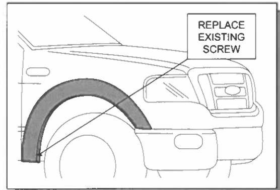
**13.** Complete installation by replacing the previously removed screw at position **F**, ensuring the Fender Flare is located over the black trim.
