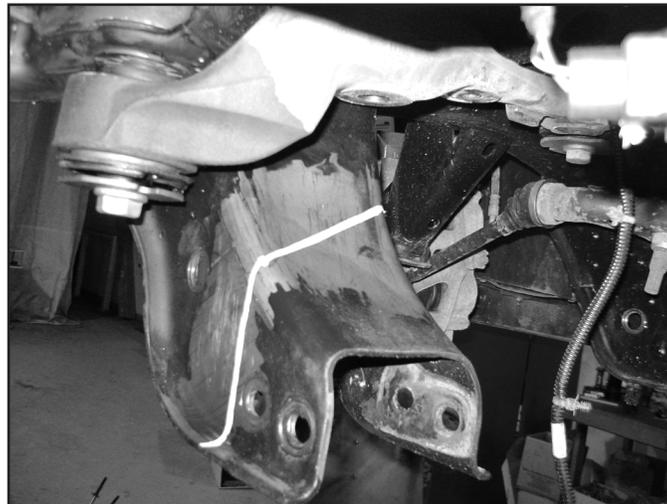
31. Using a reciprocating saw (recommended), cut-off wheel, or plasma cutter, cut the pocket along cut lines. Remove any burrs or rough edges and paint any bare metal to prevent corrosion.
