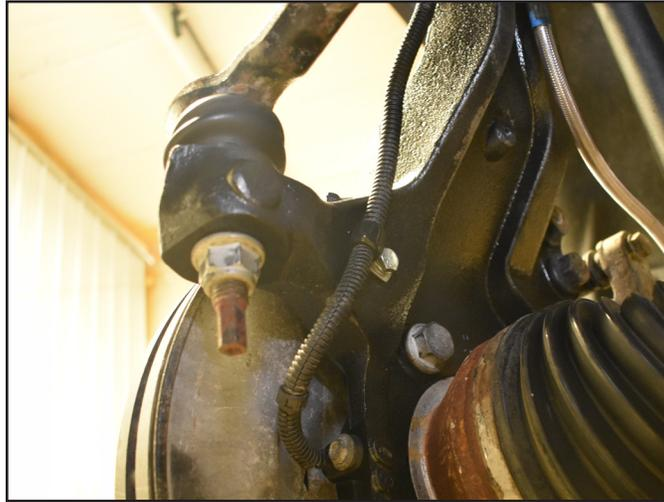
73. Install the torsion bar through the new torsion bar drop bracket, through the factory middle cross member and into the torsion bar keys in the torsion bar cross member. Do not load the torsion bars at this time. Check for clearance to the torsion bar and the middle cross member. Clearance out the middle cross member 1/4" in the area shown in Figure 50. Slide the torsion bar out for ease of access to grind the middle cross member for clearance.
