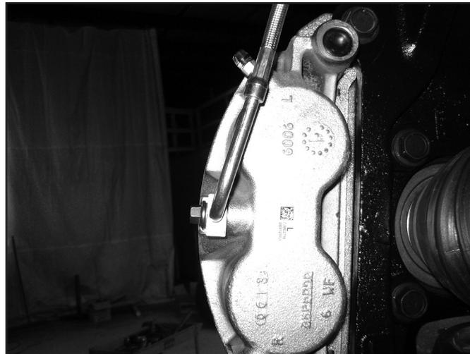
80. Remove the factory brake line from the caliper. Be sure to remove the factory crush washers as well. Place a new provided crush washer on each face of the new brake line and install on the caliper with the factory banjo bolt. Torque the bolt to 30 ft-lbs.
