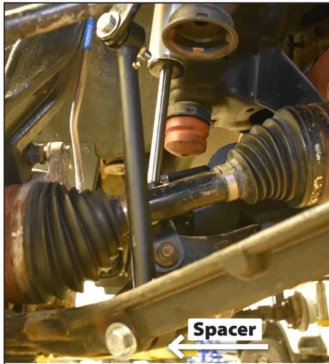
85. Attach the tie rod ends to the knuckles. The tie rod end with mount from the top down. Fasten with the original nuts and torque to 26 ft-lbs and a final pass of 85-100 degrees.
