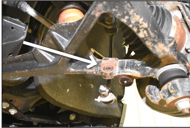
11. Disconnect the tie rod ends from the steering knuckles (Fig. 4). Remove the tie rod end nuts and save. Strike the knuckle near the tie rod end to dislodge the tie rod end taper. Remove the tie rod ends from the knuckles.
