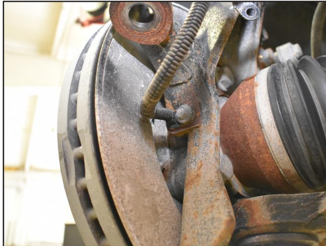
13. Remove the four bolts mounting the brake caliper assembly to the steering knuckle and hang the caliper out of the way (Fig. 8). Do not hang the caliper by the brake hose. Save mounting bolts.
