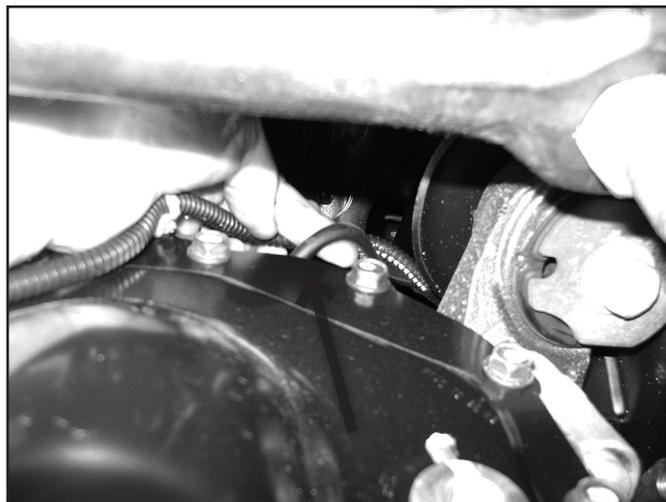
28. Loosen but do not remove all of the front differential mounting bolts/nuts. There are two nuts on the passenger's side (Fig. 20A) and three bolts on the driver's side (Fig 20B - two mount from the bottom up and one from the top down). Remove the rear-most bolt mounting from the top.
