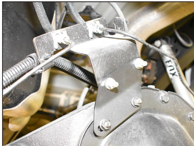
12. Install the rear ABS line relocation bracket to the differential using the factory hardware. Using the provided 1/4" hardware (BP #873) attach the rear brake line bracket to the relocation bracket (Fig. 5). Additional wire clips may need to be undone to add enough slack for the ABS lines, use the zip ties where needed.
