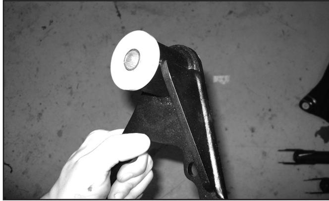
33. Locate the 4 housing bolts to be removed. Remove the four bolts, place the bracket in position and fasten with new 10mm x 40mm bolt and washers (BP #586). The bracket gusset will be toward the bottom of the differential (Fig. 23). Use thread locket on the bolt threads and torque to 59 ft-lbs.
