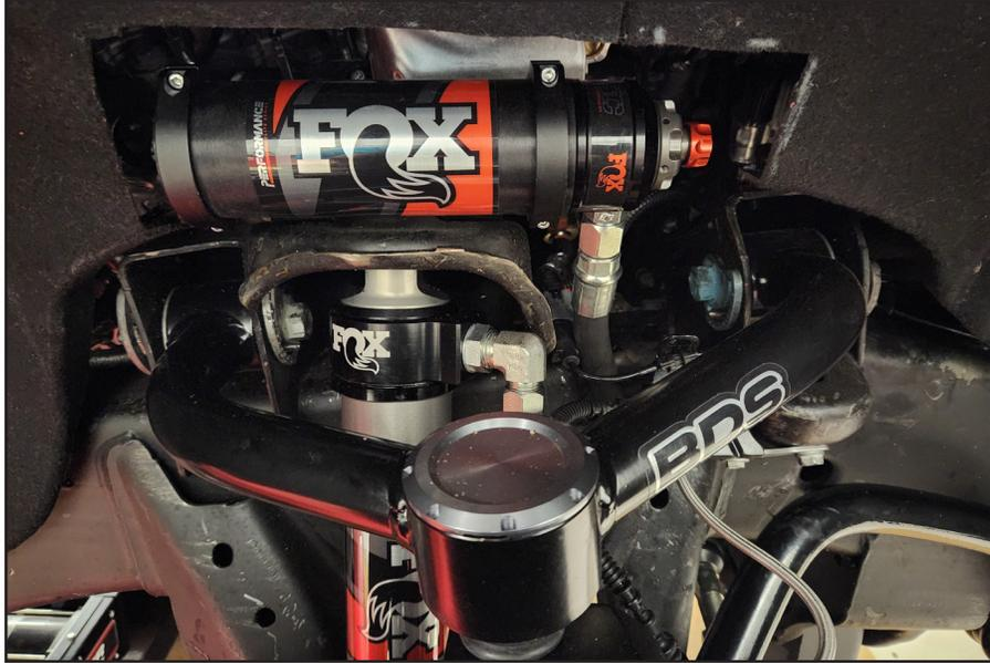
49. Install the FOX shock. To install the FOX shock, you will need to use the supplied hardware and reservoir mounting bracket. You should be using 1 reservoir bracket, 2 bolts, 2 nuts, and 4 washers per shock. (Fig. 35)
