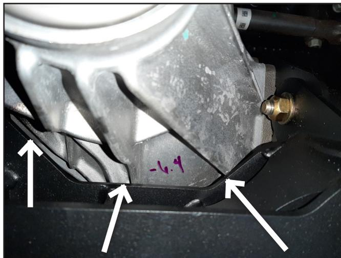
38. With the differential and rear cross member installed, tighten all the differential mount hardware. Torque the (4) 1/2" bolts to 90 ft-lbs and (1) 9/16" bolt to 95 ft-lbs.
