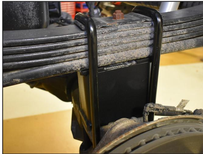
10. Repeat block installation of the driver's side.
