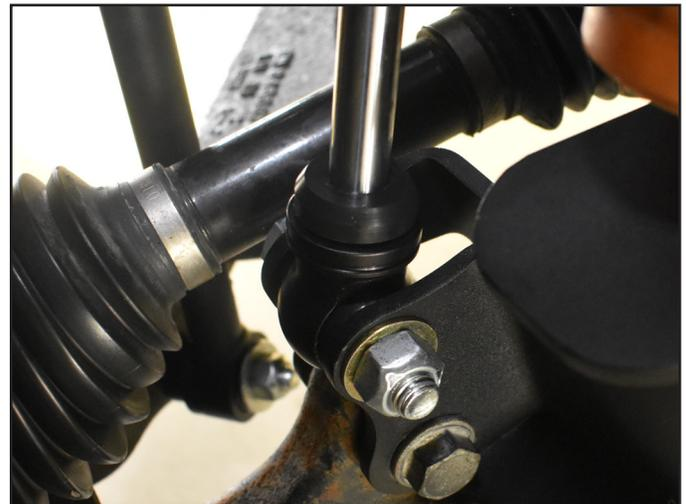
57. With the front shocks installed, torque the front shock bolt at the new torsion bar bracket to 90 ft-lbs.
