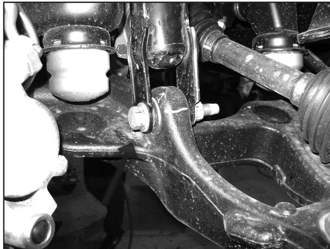
23. Remove the front and rear lower control arm bolts and remove the control arms from the vehicle (Fig. 16). Save the control arms and mounting hardware.
