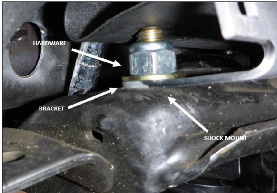
52. Swing the lower control arm up and fasten the shock to the mount on the no torsion bar drop bracket with the provided 14mm x 70mm bolt, nut, and washers (BP #587) (Fig. 38). Torque the lower shock bolt to 118 ft-lb
