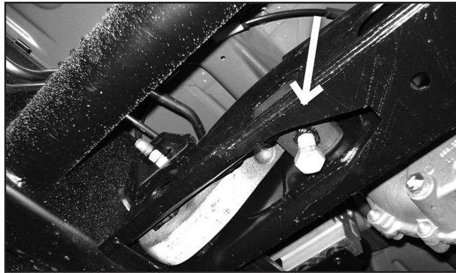
5. Unload the torsion bars but do not remove. Remove and save adjuster bolt/retainer block.
