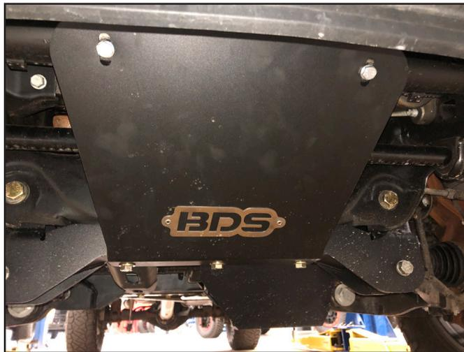
63. With the front hardware tight, remove the rear bolts one at a time and apply thread locker to the threads. Reinstall and torque to 64 ft-lbs. Torque the front factory splash guard bolts to 15 ft-lbs.
