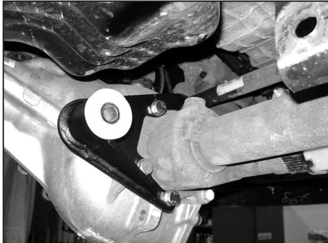
34. Locate the new passenger's side differential bracket. Bracket has a single center gusset. Install the bracket on the existing studs on the passenger's side factory bracket. Fasten with the original nuts and washers. When installed the open side of the bracket will face inward and the bracket will taper down as it goes to the rear (Fig. 24). Torque nuts to 74 ft-lbs.
