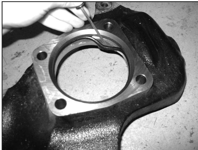
69. Locate the factory driver's and passenger's brake dust shields. They need to be modified to provided adequate brake caliper clearance. Make a cut line by following the straight edge on the caliper side of the shield all the way to the bottom edge of the shield (Fig. 46). Cut the shield along the line.
