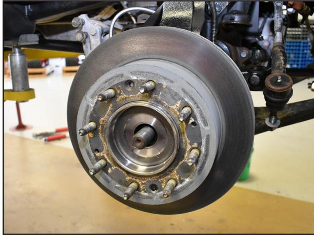
75. Tighten the CV axle nut with 34mm socket to 244 ft-lbs, then loosen 45 degrees. The final pass the CV nut should be torqued to 199 ft-lbs. Reinstall the hub dust cap.
