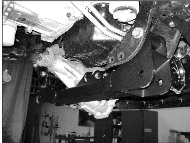
*Note: OE front differentials have varied in design with and without ribs which may interfere with the replacement rear crossmember, The ribs on the differential may need to be ground down to clear the rear crossmember. See Figure 27B.*
