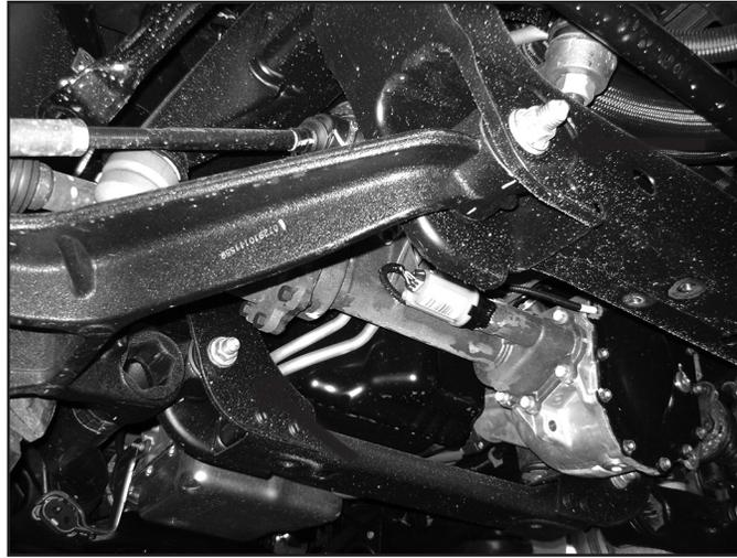
24. There are two factory bump stops per side. Remove front rubber bump stop from the frame mounts on each side. They can be removed with a pair of channel-lock pliers or by striking them with a rubber mallet. Leave the rear bump stop installed in the frame mount.
