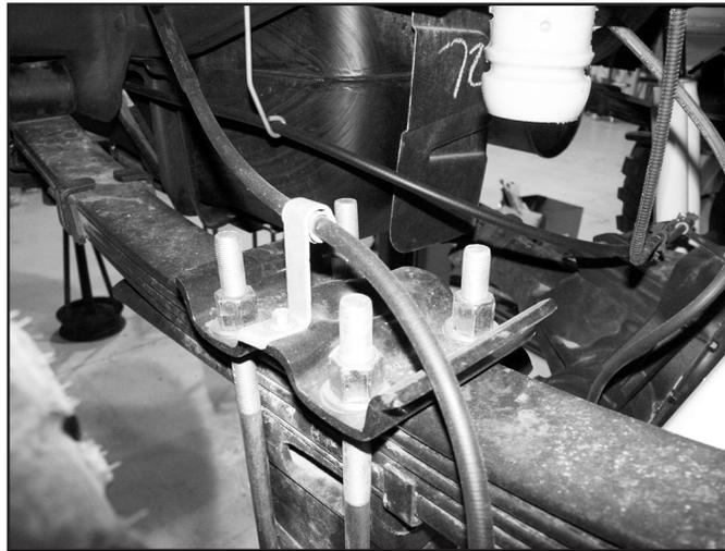
61. Reattach parking brake cable bracket to the spring plate. If more slack is needed remove the cable from the rear-most cable ring on the frame rail (Fig 16).
