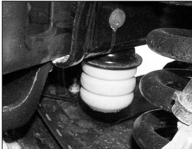
23. Position the cup on the provided bump stop extension. (4" Kit - 01000B, 6" Kit - 01001) The alignment tab on the bump stop cup will fit in the second hole in the extension.
