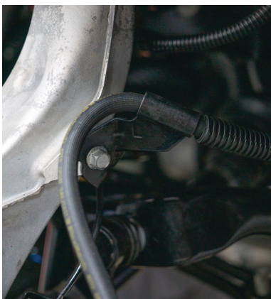
Fig. 19: Brake line bracket.
