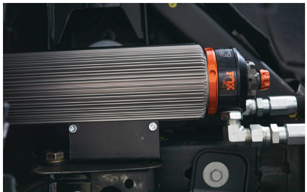
Fig. 16: Fasten the reservoir.
