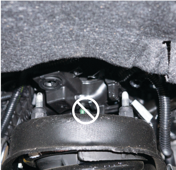
Fig. 7: Remove the three top hat nuts.
