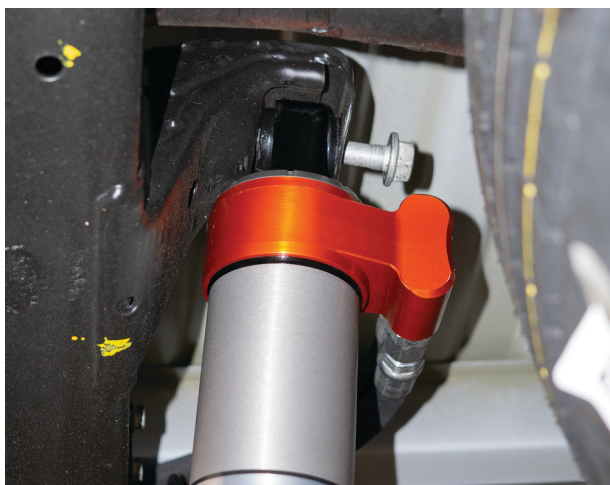
Fig. 33: The reservoir bridge faces inboard.
