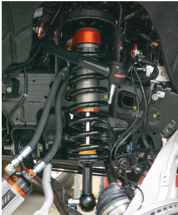
Fig. 13: Driver's side coil-over assembly is featured.
