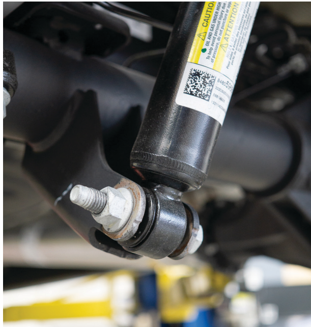
Fig. 25: Remove lower shock mount bolt.
