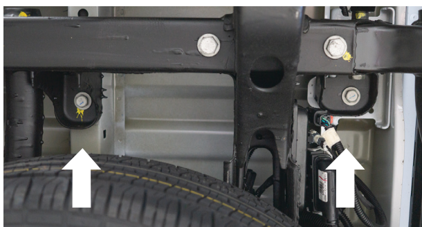
Fig. 30: Remove rear bed bolts (driver side shown).
