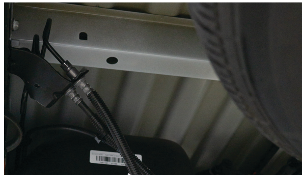
Fig. 27: Bend the brake line bracket.
