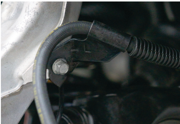
Fig. 1: Brake line bracket.
