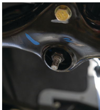
Fig. 22: Sway bar end link.
