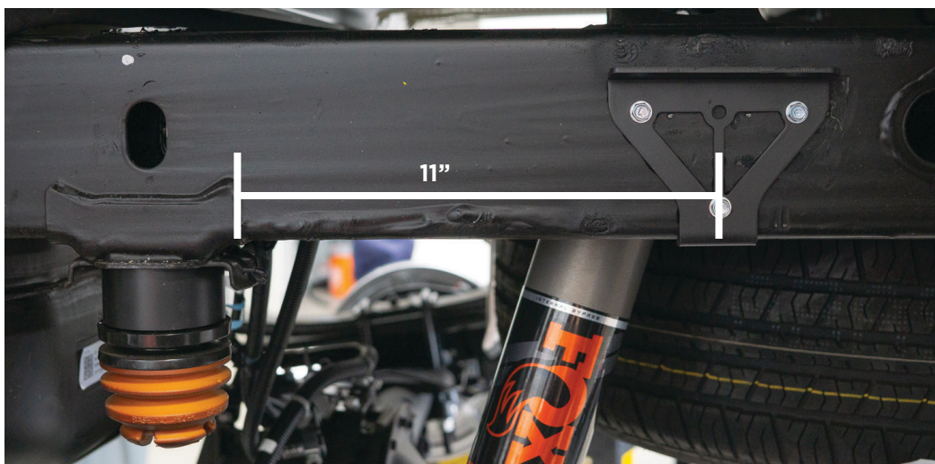
Fig. 37: Mount the reservoir bracket.
