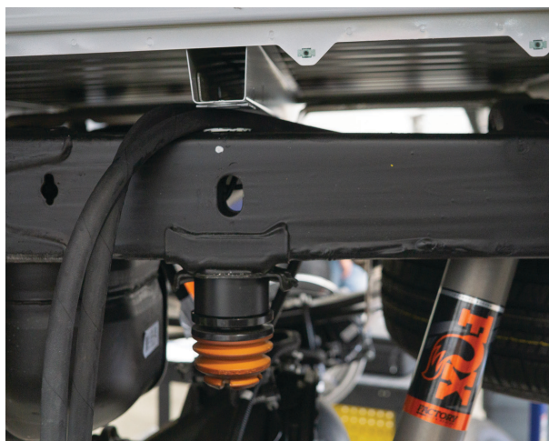
Fig. 34: Pass reservoir between the frame and bed.
