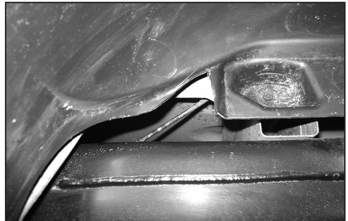
14. Remove the air bag to axle mounting nuts; 2 per side. Fig 8, 9)
