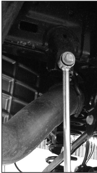
22. Remove the factory bump stops from the vehicle. (Fig 14)
