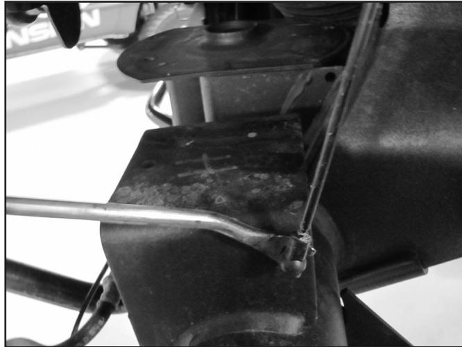
13. Disconnect the rear shocks and lower the axle, retain hardware. On the driver's side it is easiest to access the top hardware by cutting the inner fender well as shown. This trim procedure is not required but greatly aids in removal and installation of the shock (Fig 6, 7).
