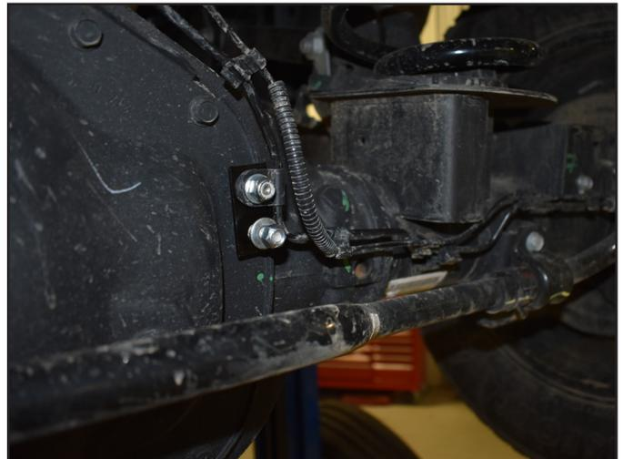
31. **5" Lift Only, E-Brake Line Brackets:** Install the driver side rear brake line bracket to reattach the e-brake to the frame. (Fig 22)
