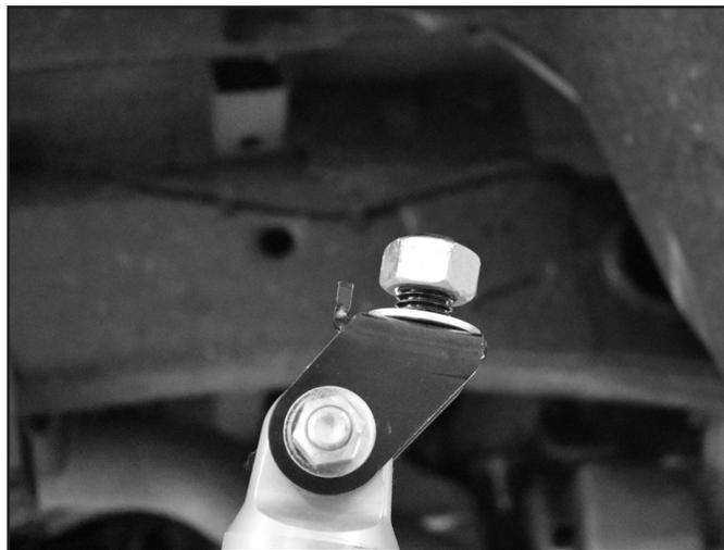
21. Grease the bushings and sleeves and install them into the sway bar links. Install the sway bar links with the new 12mm hardware. (BP 795). Tighten to 45 ft-lbs. (Fig 13)
