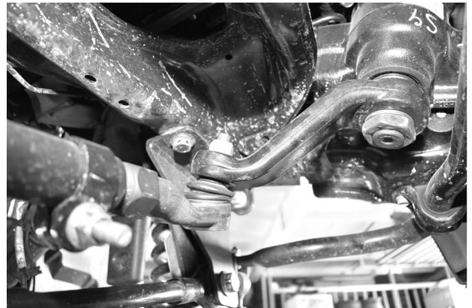
29. Install the new pitman arm, use the alignment mark made earlier. Thread locker factory nut and install with lock washer tighten nut to 332 ft-lbs. (Fig 17)
