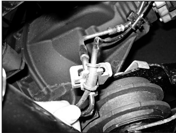
11. Detach the ABS and Central Axle Disconnect wires from retaining clips to allow for extra slack when the new coils will be installed.
