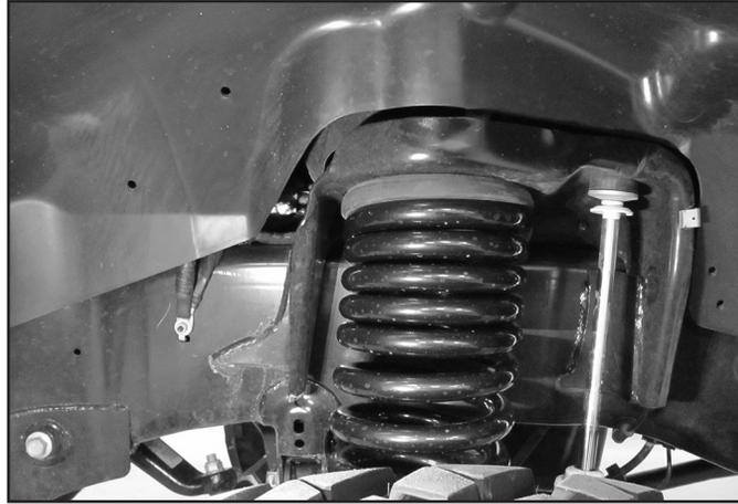
26. Attach the lower shock with factory hardware. Tighten hardware to 65 ft-lbs.
