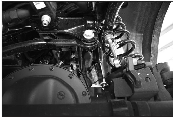
3. Raise the front of the vehicle and support the frame rails with jackstands. Do not support the vehicle by the radius arms, they will be removed during the installation.
