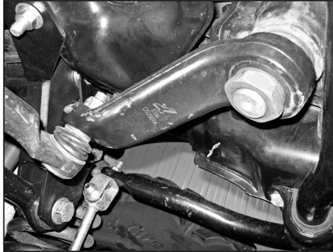
31. Disconnect the brake line bracket from the frame (Fig. 18 Driver side). Reattach the factory brake line bracket to the axle with factory hardware, torque to 10ft-lbs. slightly bend the factory axle bracket to create more slack in the brake line with a pliers or small adjustable wrench.
