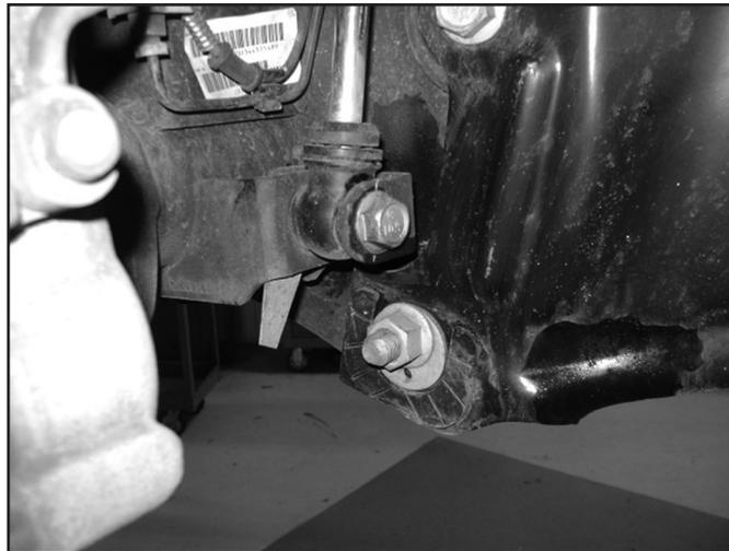
14. Lower the axle and remove the factory coils. Use care not to overextend any brake line, ABS, or CAD wires.
