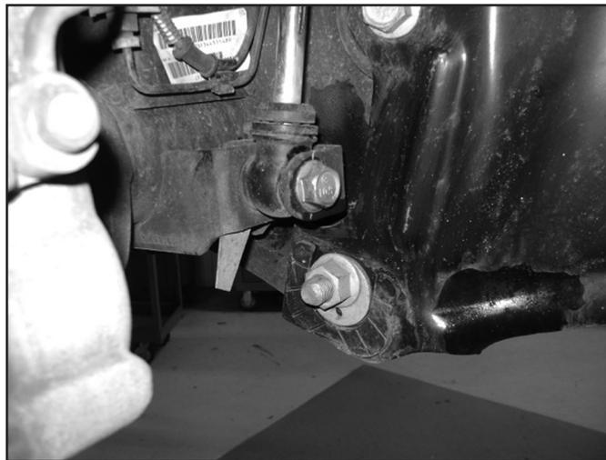
14. Lower the axle and remove the factory coils. Use care not to overextend any brake line, ABS, or CAD wires.
