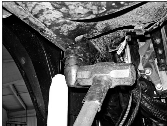
20. Grease new replacement bump stops and raise axle to press the bump stops into position. These will be a tight fit. It is easiest to lift the axle with a jack to compress the bump stops into position. (Fig. 10)
