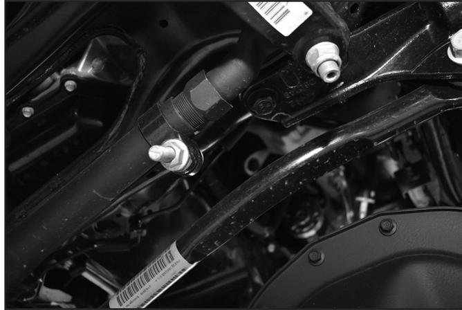
8. Disconnect the drag link tie rod from the pitman arm, do not damage the tie rod boot. Mark the orientation of the pitman arm and remove the pitman arm from the sector shaft. (Fig. 3)
