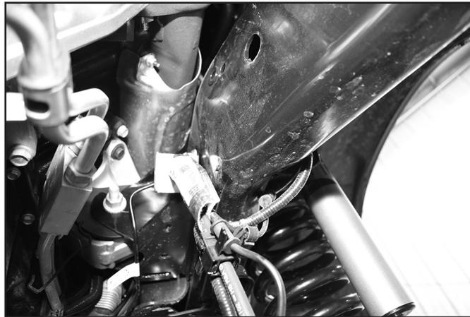
33. Install the sway bar drop brackets with factory hardware to the frame. The flat side of the bracket will face "out" and the brackets will offset the sway bar slightly forward. Attach the sway bar to the drop brackets with 3/8" hardware (Bolt Pack 422), tighten factory hardware to 43 ft-lbs and 3/8" hardware to 37 ft-lbs. (Fig. 16, 17)
