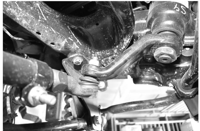
29. Install the new pitman arm, use alignment mark made earlier. Thread Locker factory nut and install with lock washer tighten nut to 332 ft-lbs. (Fig 13)
