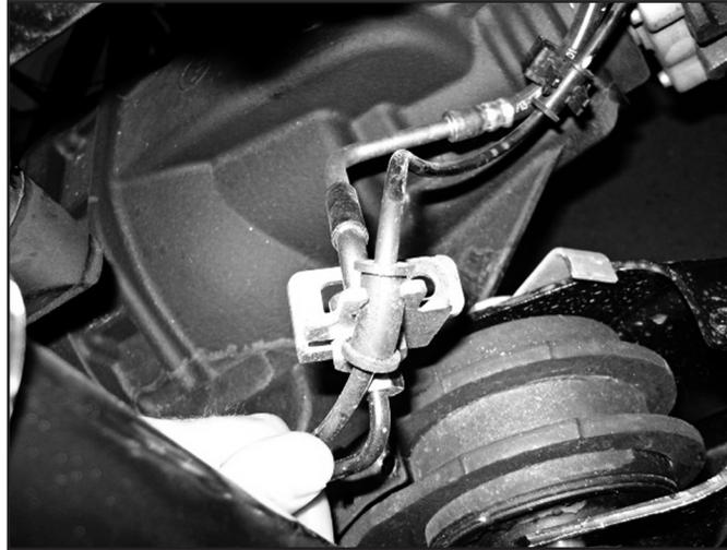
11. Detach the ABS and Central Axle Disconnect wires from retaining clips to allow for extra slack when the new coils will be installed.
