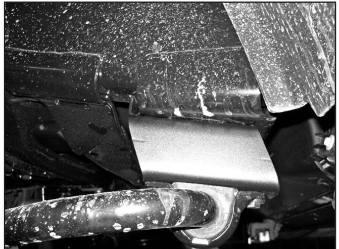
34. Reconnect the sway bar links with the factory hardware, torque to 60ft-lbs
