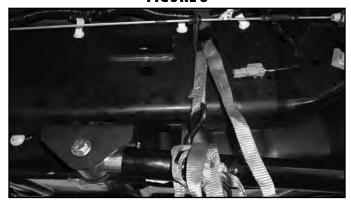
20. While holding the bracket in place, use the holes and center of the two slots in the frame bracket as a template, mark the location to be drilled on the frame. Since a nut tab is used, **it is important that the holes are centered on the slots** (see Figure 10). Use the template at the end of the instructions to create a precise location to drill the holes. Lower the Recoil Traction Bar from the frame rail.
