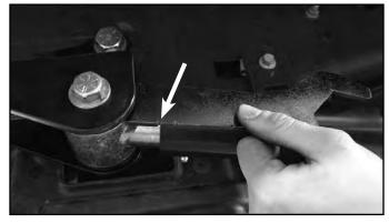
37. Utilize the Jam Nut Wrench to set a desired force setting (Minimum of the First Level). Depending upon suspension setups, different spring preload may need to be tried to find a good setup to reduce axle wrap. After the desired force is set, lock off the jam nut with the two provided Jam Nut Wrenches and repeat this process on the other Recoil Traction Bar.
