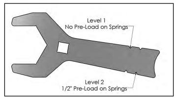
36. Utilizing the Levels on the wrench, spin the Recoil Traction Bar either clockwise to add more force into the dual coil springs setup to reduce axle wrap, or loosen the Recoil Traction Bar by spinning it counter clockwise in order to reduce the input the Recoil Traction Bar has on the suspension system.
