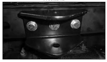
25. Reattach the Recoil Traction Bar to the frame bracket with the 9/16" x 4-1/2" bolt, 9/16" nut, and two 9/16" SAE Washers, leave hardware loose. Attach the new skid plate support bracket (03415) on the inside of the frame bracket with the 9/16" hardware. The bracket should support the bottom of the fuel tank skid plate.
