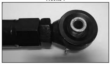
13. Attach the Recoil Traction Bar to the axle bracket with a 9/16" x 4" bolt, 9/16" nut and 9/16" SAE washers from Bolt Pack 964. Install the Recoil Traction Bar so that the Forged Flex End (A171) is mounted to the axle bracket. Leave mounting hardware loose at this time
