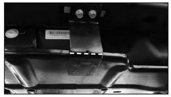
17. Remove the two bolts that are attached to the upper part of the fuel tank skid plate support that was just cut. Remove the two J-nuts from the frame rail.
