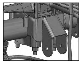
10. Locate two of the 1/2" U-bolt and install around the axle and up through the sleeves in the axle mount bracket (02886). Using the 1/2" fine thread nut and 1/2" SAE washer from Bolt Pack 962, tighten the U-bolts so that the axle mount clamps around the axle. The axle mount bracket should be parallel with the leaf spring perch. Tighten the 1/2" fine thread hardware to 45 ft-lbs.
