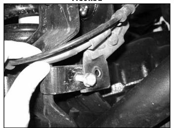
8. Disconnect the sway bar links from the sway bar clevis bracket which is included in the long arm kits (Fig 3).
