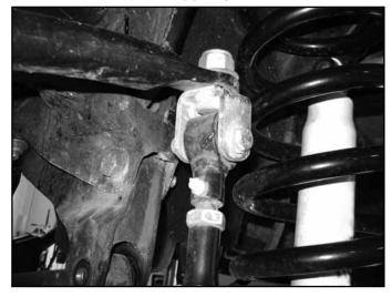
9. Disconnect the drag link from the pitman arm (retain nut), disconnect the trackbar from the frame bracket. (Fig 4)
