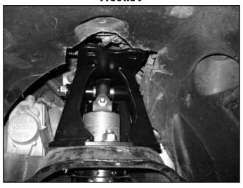
23. Attach the reservoir mount to the upper coilover mount with ½" hardware with washers and loc nuts. Tighten to 65 ft-lbs. Attach reservoir to the mount with hose clamps included with Fox Coilover Box Kit. (Fig 10a, 10b)
