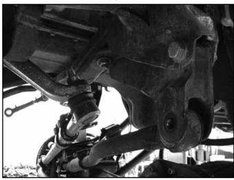
10. Vehicles WITHOUT transfer case indexing ring kit installed or gas model trucks: Disconnect the driveshaft from the front axle. Note: It may be necessary to heat the front axle yoke to get the loc-tite to break free. Retain all hardware. (Fig 5) (Diesel trucks w/ indexing ring kit installed may skip this step)
