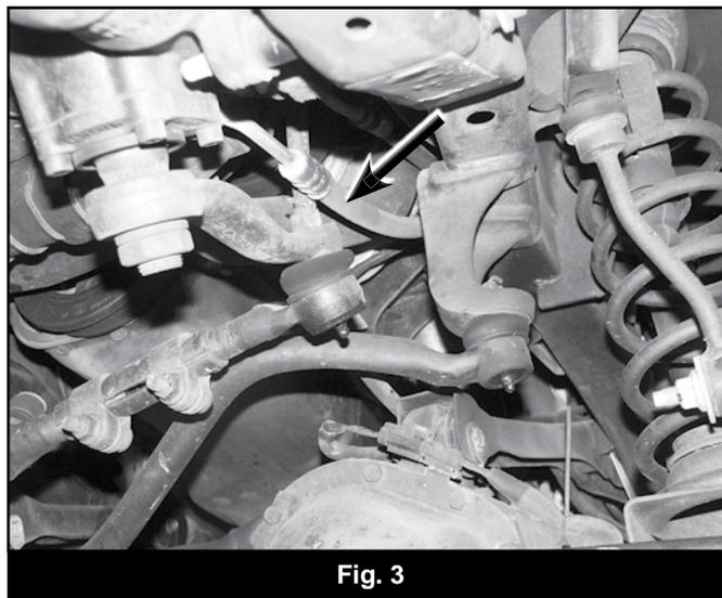
10. Remove the driver's and passenger's side coil spring retainer clips located on the back side of the axle coil seat. Save clips and bolts.
