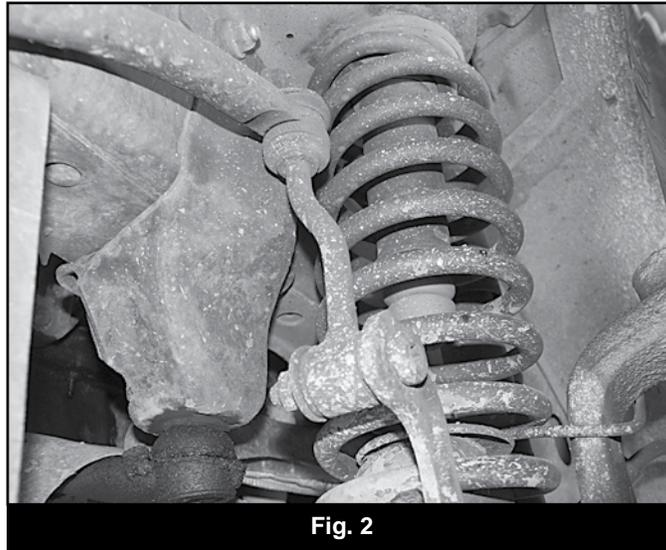
8. Disconnect the sway bar links from the axle. Remove the nut and the sway bar link from the bolt (Fig 2). Some early models will require a T55 torx socket to hold the bolt from rotating. Later models used a bolt with a serrated neck that is pressed into the bracket so it will not rotate. Save axle mount hardware.
